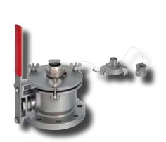
The **HERMetic Sampler GT4** is dedicated for closed sampling of liquids and where more than 0.5 litre of liquid is needed. Its gas tight construction avoids a pressure release from the tank and exposure to fumes during opera-
