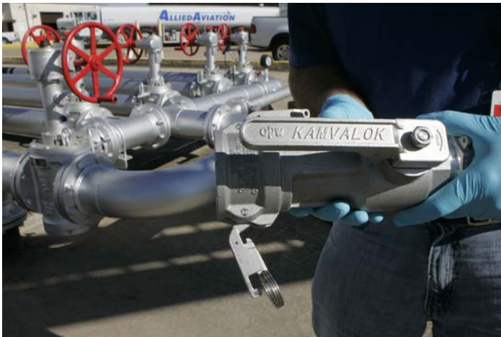
Allied Aviation received the prestigious Silver Nozzle Award for Organizational Excellence from the National Petroleum Management Association in 2007. A key component of its safer system, was the incorporation of the Kamvalok® Dry Disconnect System from OPW Engineered Systems, Lebanon, OH.
