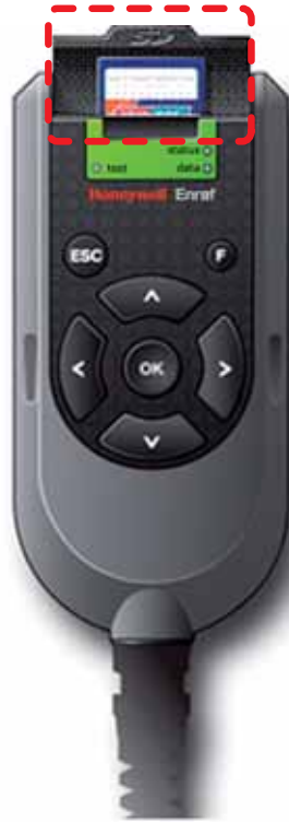
FIGURE 5-6 SD card location in LAD (lid opened)
