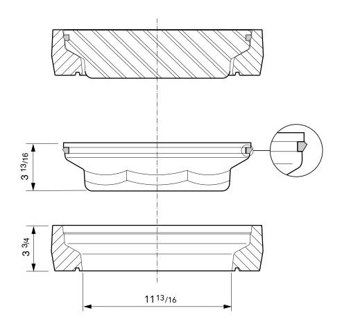
12" diameter flat sealed composite cover with "Grounding Point" ID logo and composite frame.
