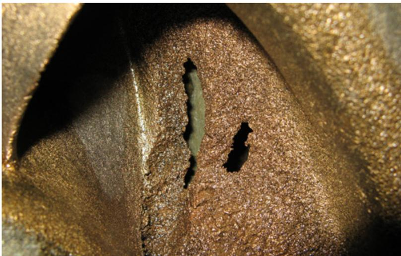
Hole in impeller blade
