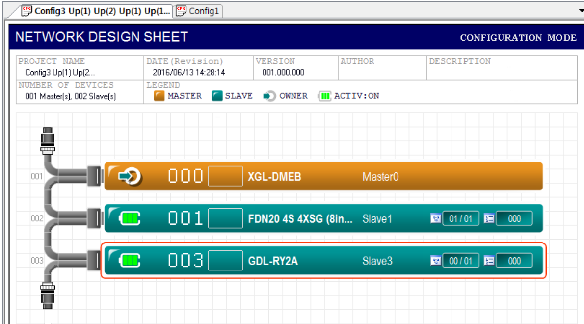
[Figure 5.35.6] Example of screen restored to the configuration mode by the completion of diagnostic mode
