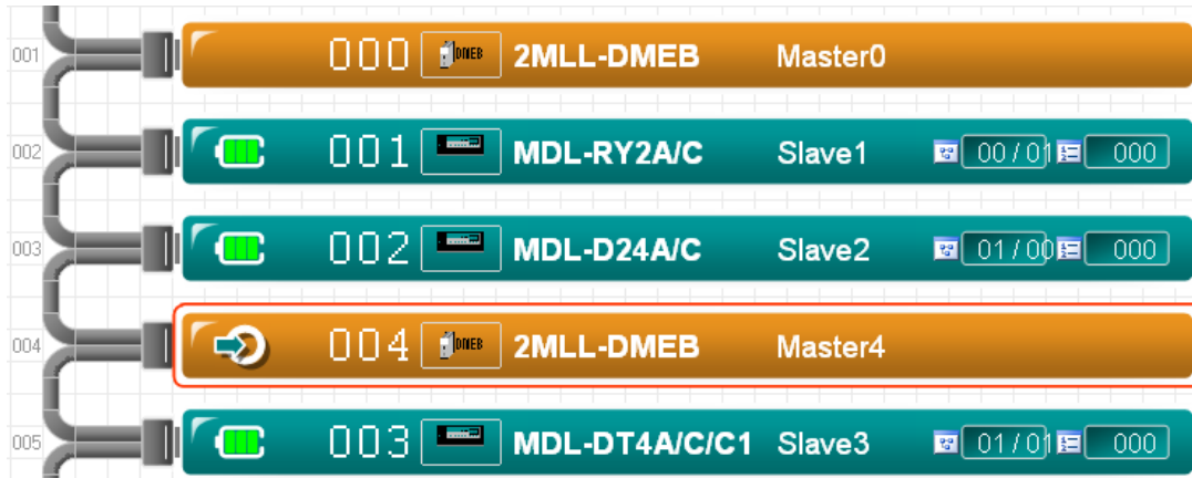
[Figure 5.26.5] Screen of the case where the slave device with address 2(which belongs to the master device whose address is 0) is selected
