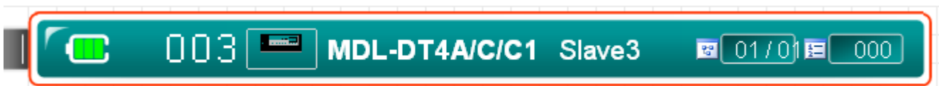
[Figure 5.26.9] Slave device in case Activate Device item is set to “Activate”
