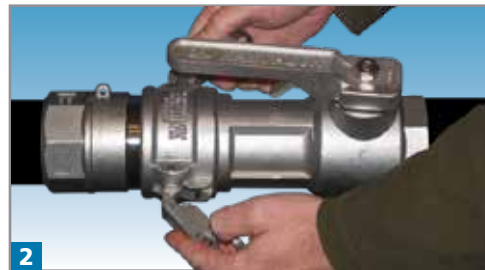
2 Cam Arms Lock Coupler and Adaptor Together
