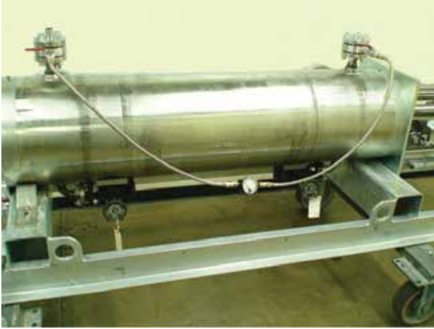
Figure 4-1: Static Leak Detection Set-up
