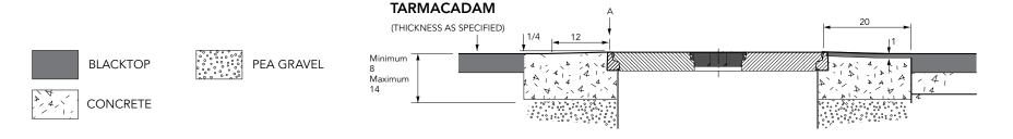
40" dia. watertight flat sealed composite cover and frame with removable central dip cover (10" dia.)
