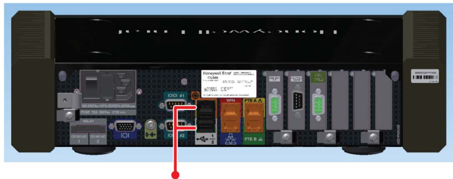
FIGURE 1-12 CIU 888: USB ports located at the back
