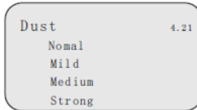
When the liquid level fluctuates greatly or the dust is large, the position and intensity of the wave peak are unstable.
