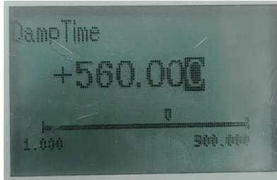
To damp process-dependent measured value fluctuations, set an integration time of -999.999 ... +999.999 s in this menu item. Default setting is 60s.
