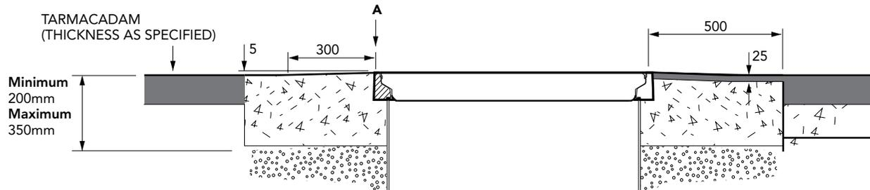
900mm dia. watertight flat sealed composite cover and frame, with a central dip port cover.
