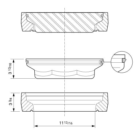
FL120 Monitoring Well - 12" diameter flat sealed composite cover with "Do Not Fill" ID logo and composite cover.
