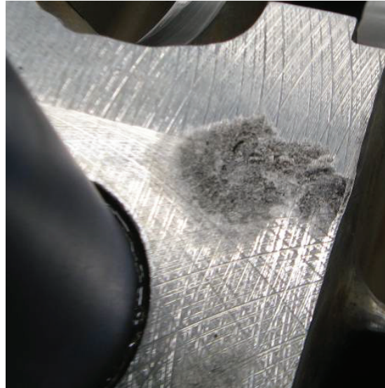
Figure 2 – crevice corrosion on split flange
