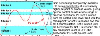
See Automatic Tuning section 4 for tuning the PID sets.
