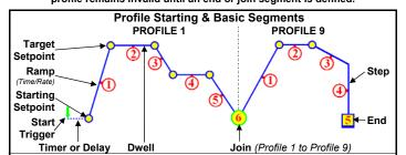
ollowing a Start Trigger, profiles can start immediately, or if enabled after a delay or at a specified day & time (Recorder only).
