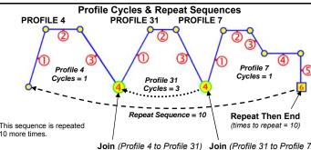
profile can be made to run itself 1 to 9999 times or continuously using the Profile cycles setting. A profile ending with Repeat Then End will run the entire sequence of profiles again 1 to 9999 times or continuously.
