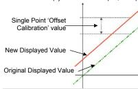
This example shows a positive offset value E.a. if the process displays 27.8 when it should read 30, an offset of +2.2 would correct the displayed value to 30. The same offset is applied to all values, so at 100.0 the new value would be 102.2.
