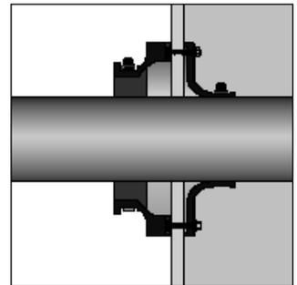
**Note:** When installing DEB-0200s with FlexWorks Pipe, you must install the entry boot prior to coupling the pipe.
