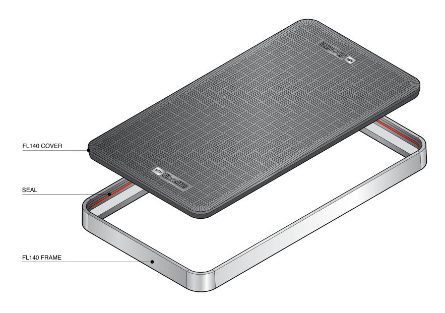
1400mm x 700mm flat sealed composite cover and aluminium frame.
