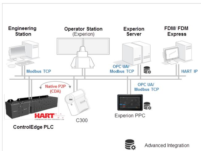
Figure 4. ControlEdge PLC, Experion and Experion PPC Integration
