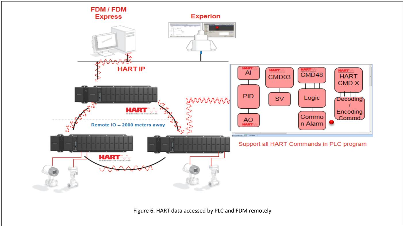
Figure 6. HART data accessed by PLC and FDM remotely
