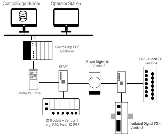
Figure 9 – Multivendor EtherNet/IP device and I/O module connectivity
