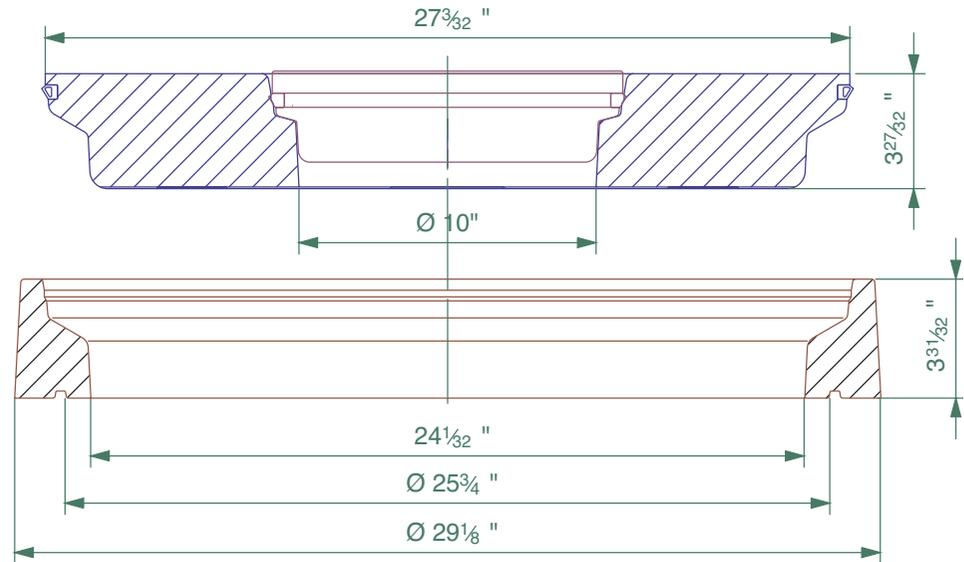
24" diameter flat sealed composite cover with a central port cover and composite frame.
