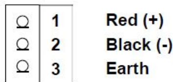
Figure 5: Wiring an External DC Supply
